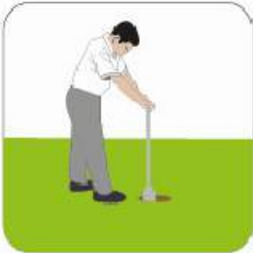
Drill hole using Auger
